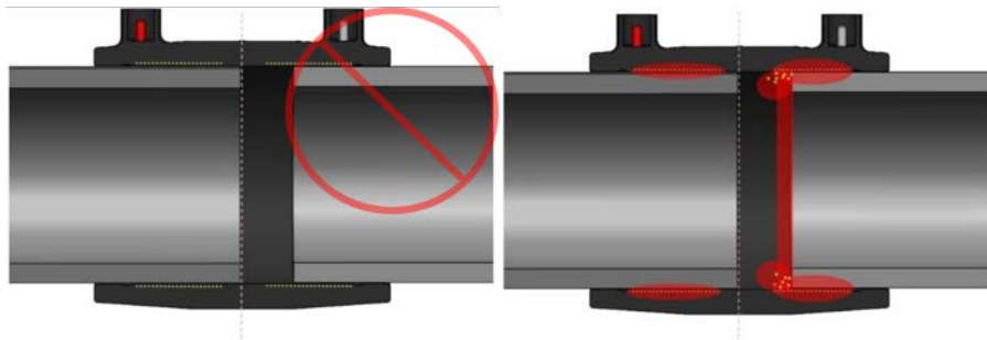
Figure F-a: Short Stab - Incorrect Assembly
